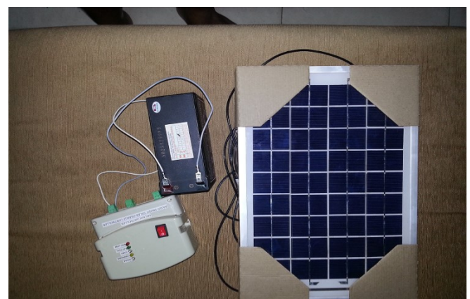
Fig-8 (a): Charge controller, Battery and Solar panel
