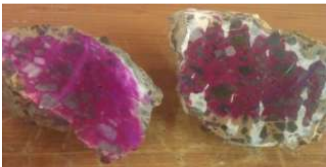
Fig – 8: Carbonation test and change of colour
