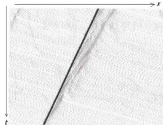
Fig-4: Space-time diagram of NaSch model with v_{\max} = 5 , p = 0.4 and a supercritical density \rho = 0.2 . The added line indicates the front of traffic jams.
