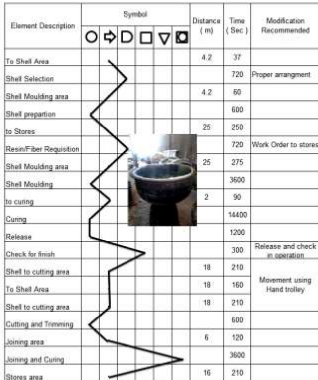
Chart -1: Process Flow Chart-Shell Moulding
