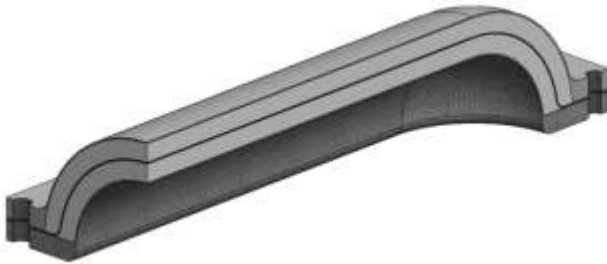
Fig 2 Cross Section of 'C' Sandwich Radome
