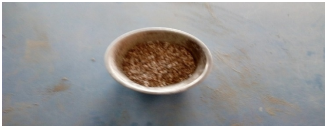
Fig-6: Tile powder passing 2.36 IS sieve
