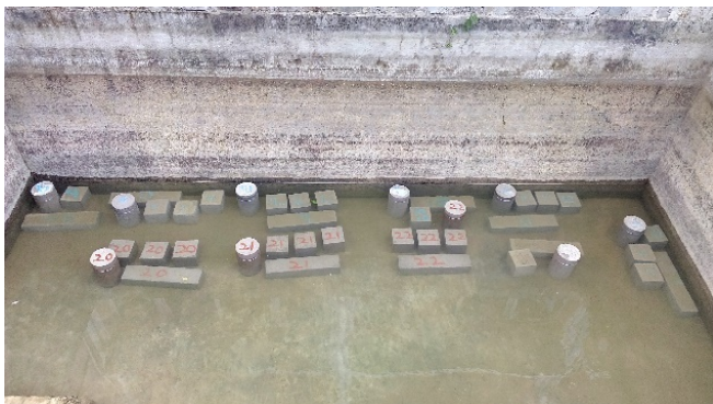
Fig-8: Curing of specimens
