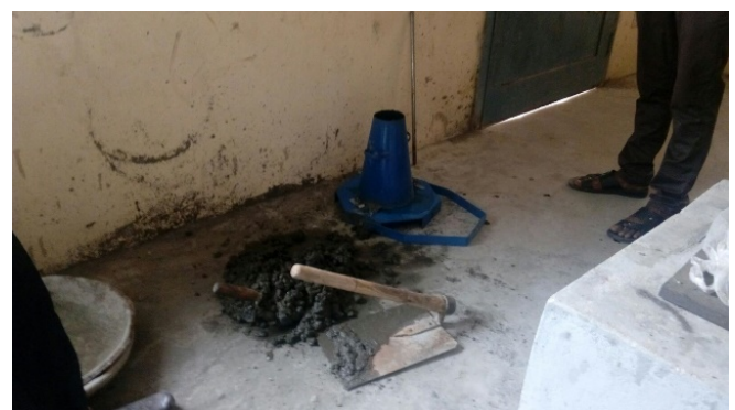
Fig-7: Mixing of concrete
