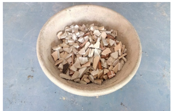
Fig-5: Tile chips obtained after sieving in IS 20mm sieve
