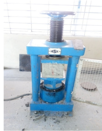
Fig-9: Compression testing of cubes
