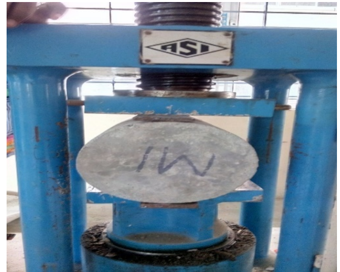
Fig-10: Split Tension test
