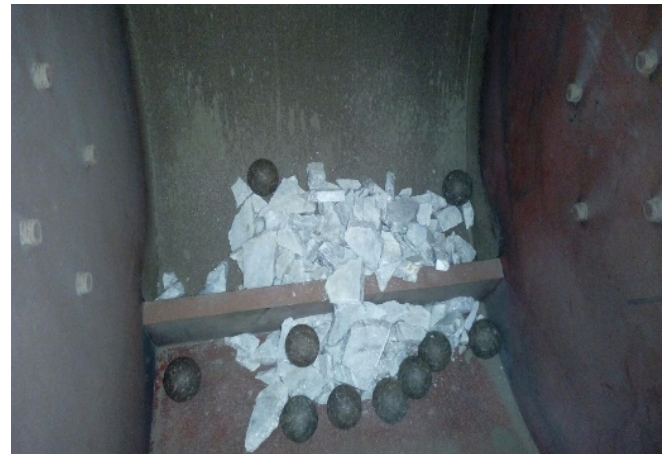
Fig-3: Marble before crushing
