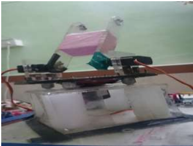
Fig 3.2.4 lower link placed in the supports
