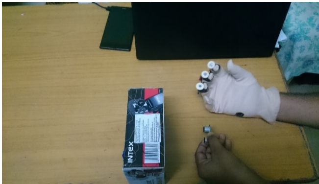
Fig 4.2.6 Experimental setup for 15cm distance showing all three motors vibrating
