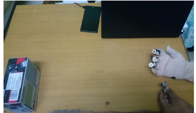
Fig 4.2.3 Experimental setup for testing haptic feedback system the ultrasound sensor in hand indicating position of electrode and the box indicating the workpiece
