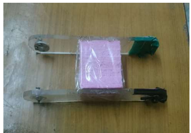
Fig 3.2.3 the lower link with thermos foam in between used as a spacer
