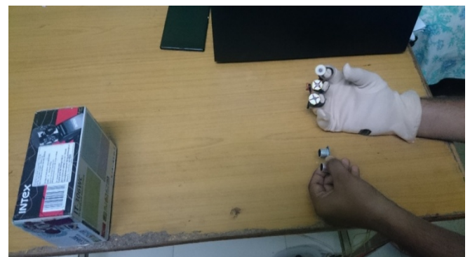
Fig 4.2.4 Experimental setup for 45cm distance showing only one motor vibrating
