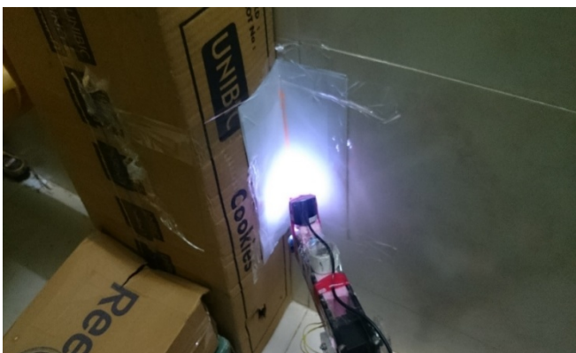
Fig 4.1.2: the robotic end effector performing welding
