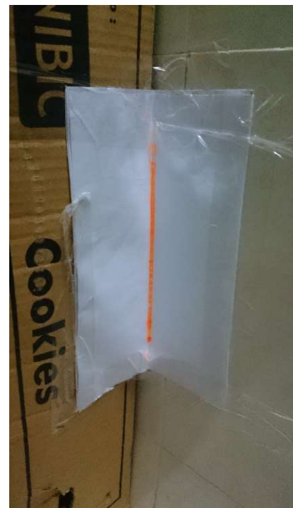
Fig 4.1.4 the weld bead after welding process indicated by the orange line
