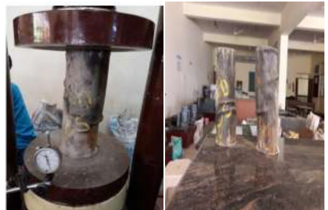
Fig-5: Testing of specimen using CTM & Specimen after failure
