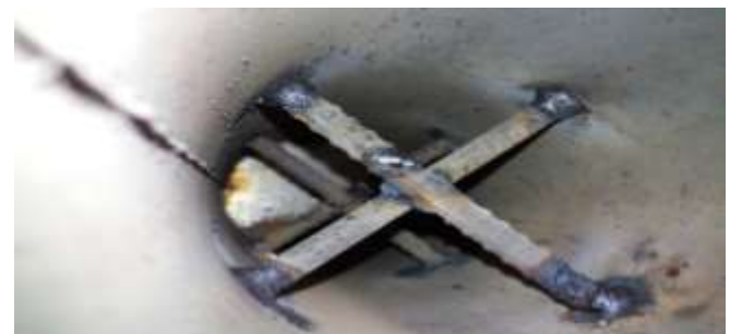
Fig-3: Double stiffened specimen
