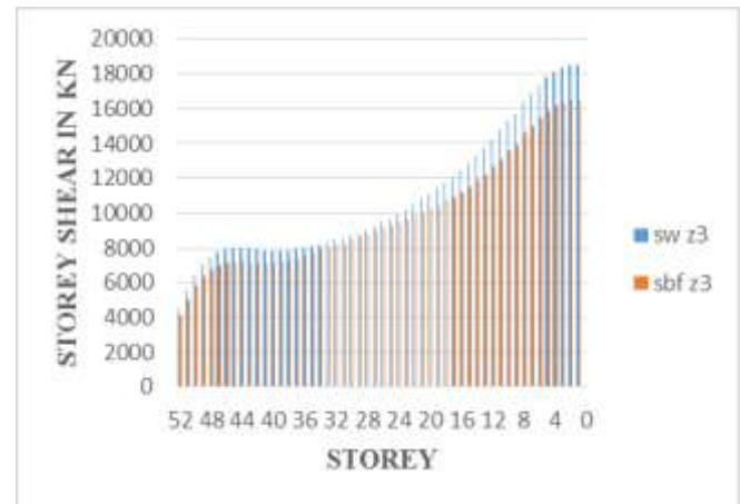
Fig 14: Storey shear vs. storey for sw z3 and sbf z3 due to response spectrum loads
