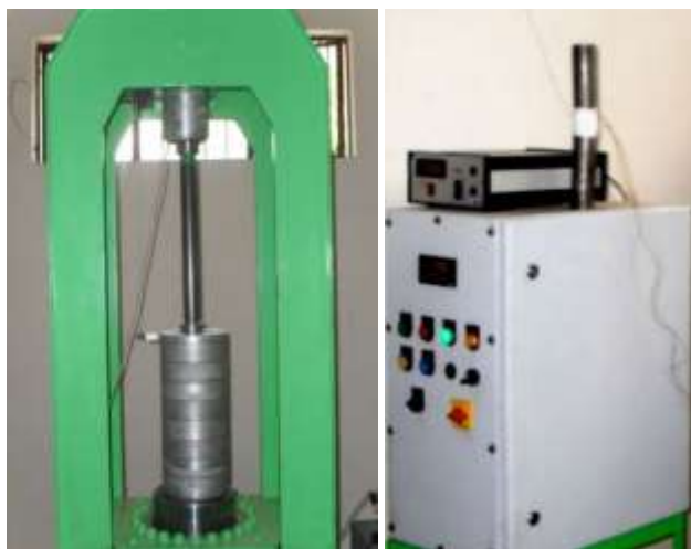
Fig 6: 200 Ton Capacity Hydraulic Monotonic Loading Machine
