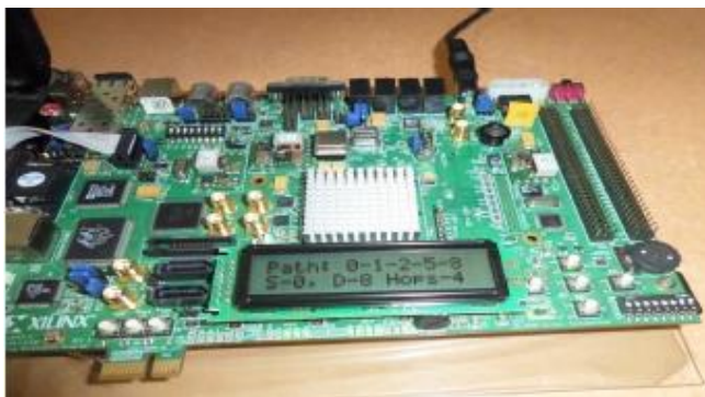
Figure 17: FPGA implementation of packet routing in NoC without faulty Link
