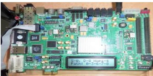
Figure 18: FPGA implementation of packet routing in NoC with faulty Link
