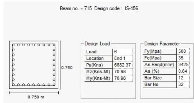
**Fig 5-** Concrete design of Column 715 in CASE 2
