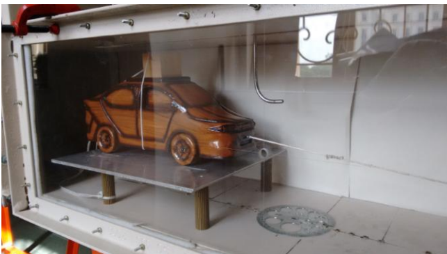
Figure 3: Car model on rectangular plate inside wind tunnel Following table 1, gives the velocity, drag force, projected area and drag coefficient for the cases considered for this study.
