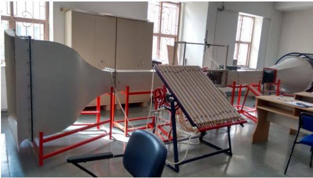
Figure 2: Wind tunnel set up with multitube manometer
