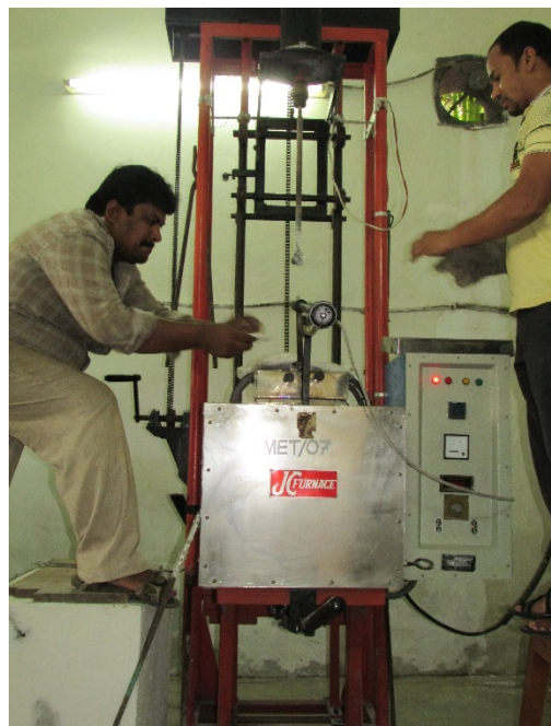
Fig-1: Real photo of used vertically aligned pit type bottom poured melting furnace
