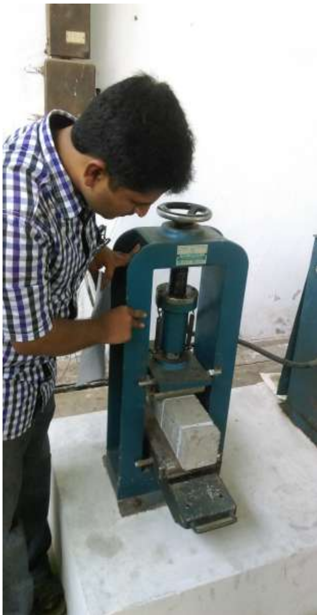
Fig.3 :Testing of GPC Prism
