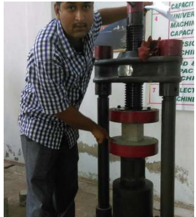
Fig.1 : Testing of GPC cubes
