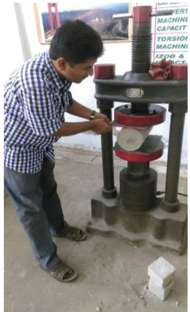
Fig.2: Testing of GPC cylinder
