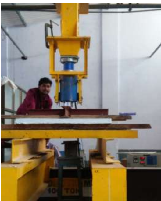
Fig :11 Testing of slab on loading frame
