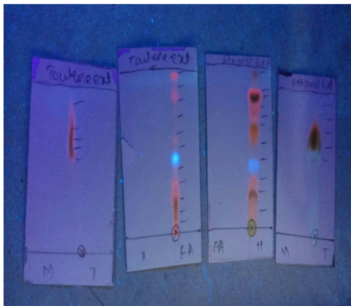
Fig.2: Fluorescent spots observed under UV light for toluene and ethanol extract
