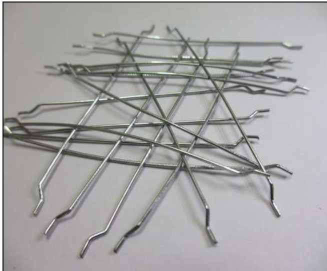
Figure 1: Hook end steel fiber
