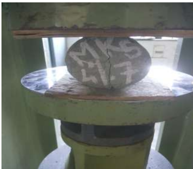
Figure 4: Crack pattern for metakaolin blended sifcon cylinder
