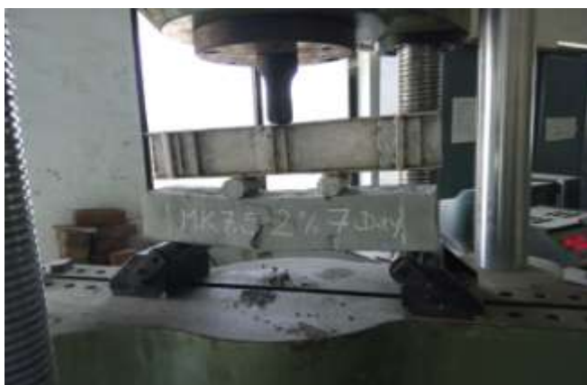
Figure 3: Crack pattern for Metakaolin blended SIFCON beam
