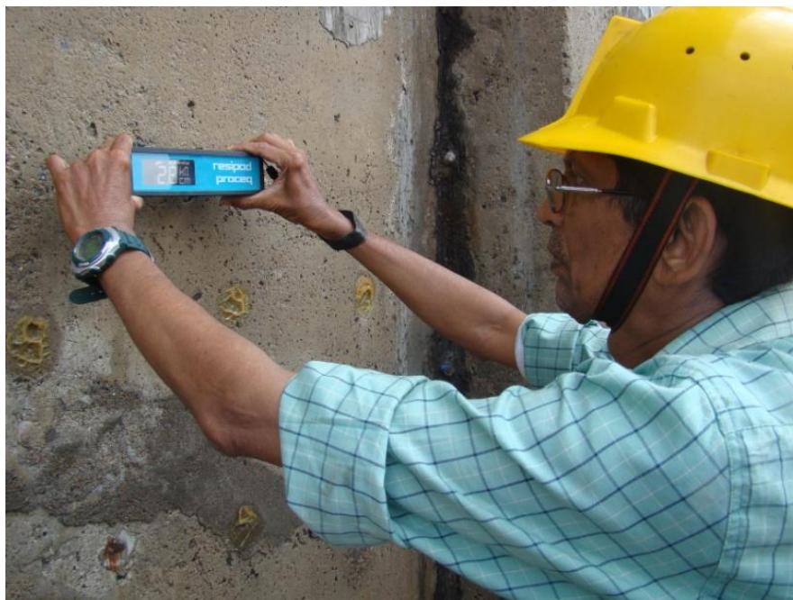
Fig. 4 Typical resistivity measurement
