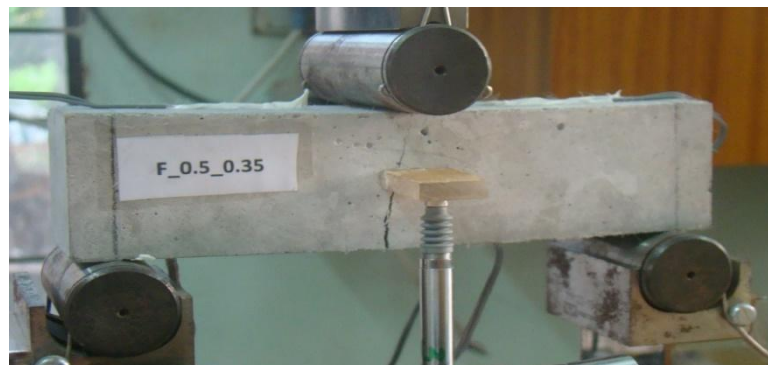
Figure 3 – Fiber incorporated specimen with 0.35 w/c (after reaching first crack strength) being subjected to three point bending.
