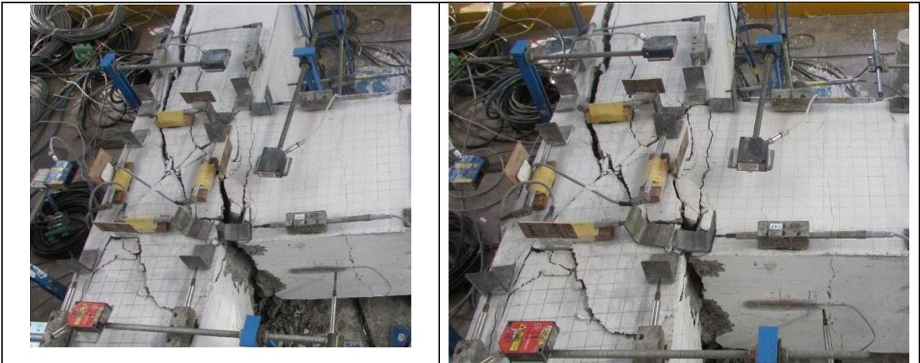
**Fig 4b** Crack pattern at +5.88%(left) and -5.88%(right) drift ratio –SP2
