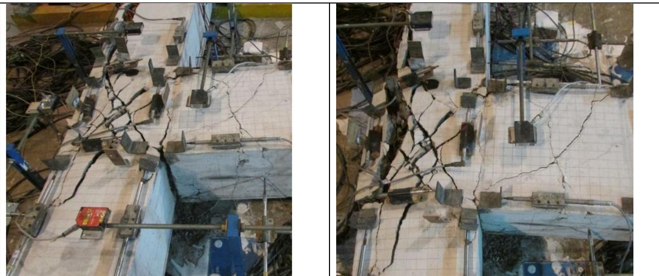
**Fig 5** Crack pattern at +7.05%(left) and -7.05%(right) drift ratio –SP3
