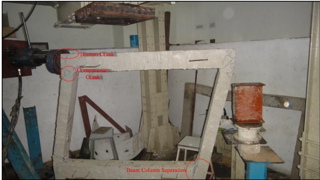
Figure 7: Failure in bare RC Frame
