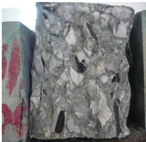
Fig-12: Interfacial transition zone failure of CWAC after testing
