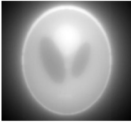
Fig -6: Image reconstructed using simple back projection Method.
