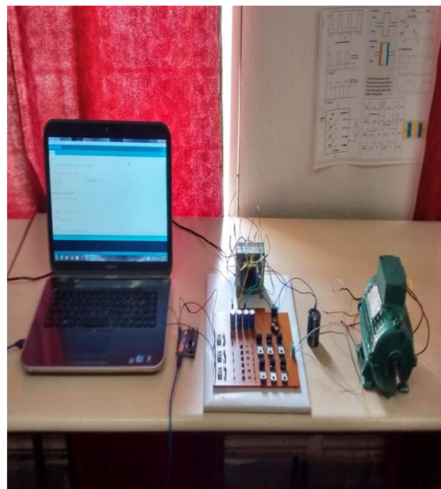
Fig 11 Hardware setup of three phase inverter fed to three phase induction motor
