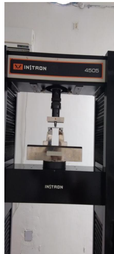
Fig.4: Test for Flexural Strength
