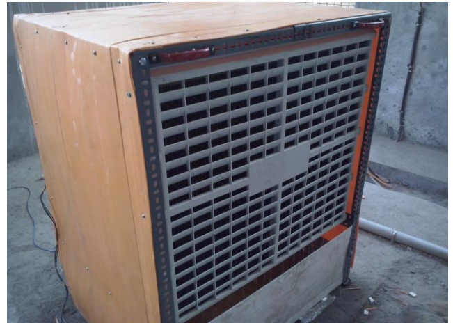
Fig 2: Fabricated evaporative cooling system
