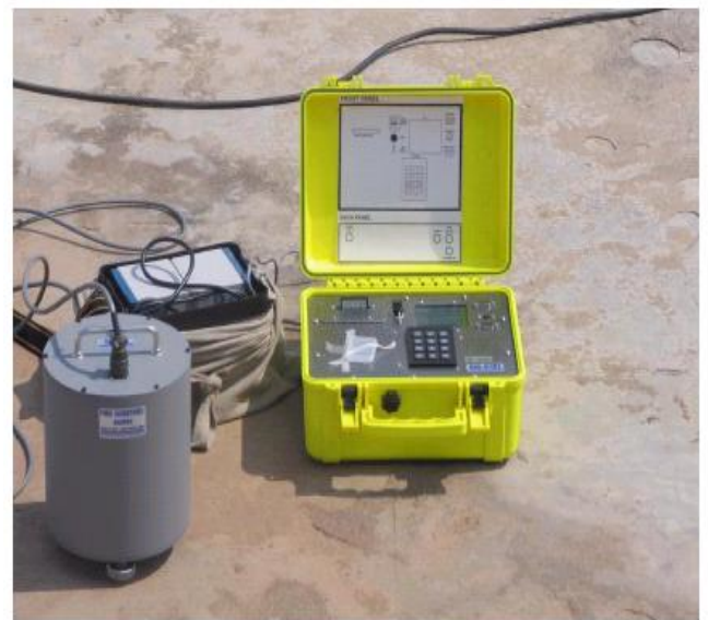
Fig -1: Figure-1: Data acquisition system and Sensors of a typical portable AVT equipment
