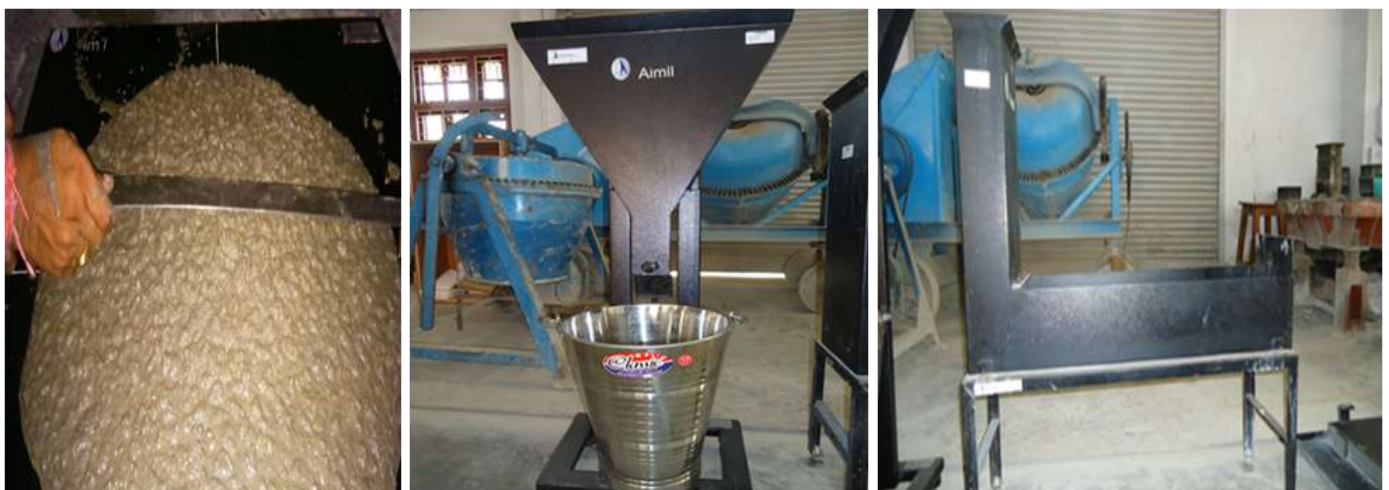
Figure-3: (A) Slump flow test, (B) V-Funnel test, (C) L-Box test
