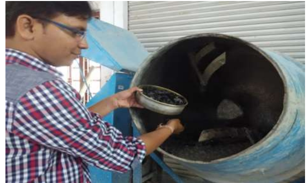
Figure-2: Preparation of SCC Mix
