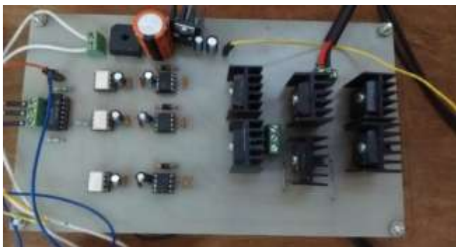
Fig-11: Inverter Circuit
