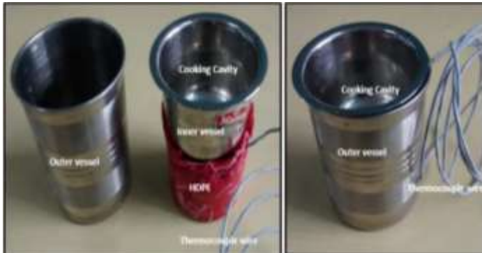
Fig -7: Images of Assembly of thermal storage device.
