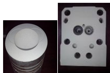
Figure 2: piston crown and cylinder head coated with Magnesia Stabilized Zirconia (Mg-PSZ)
