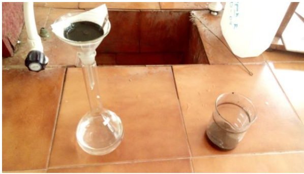
Figure 2.1: Extraction fluid filtered through 0.6-0.8µm glass fibre filter paper.
