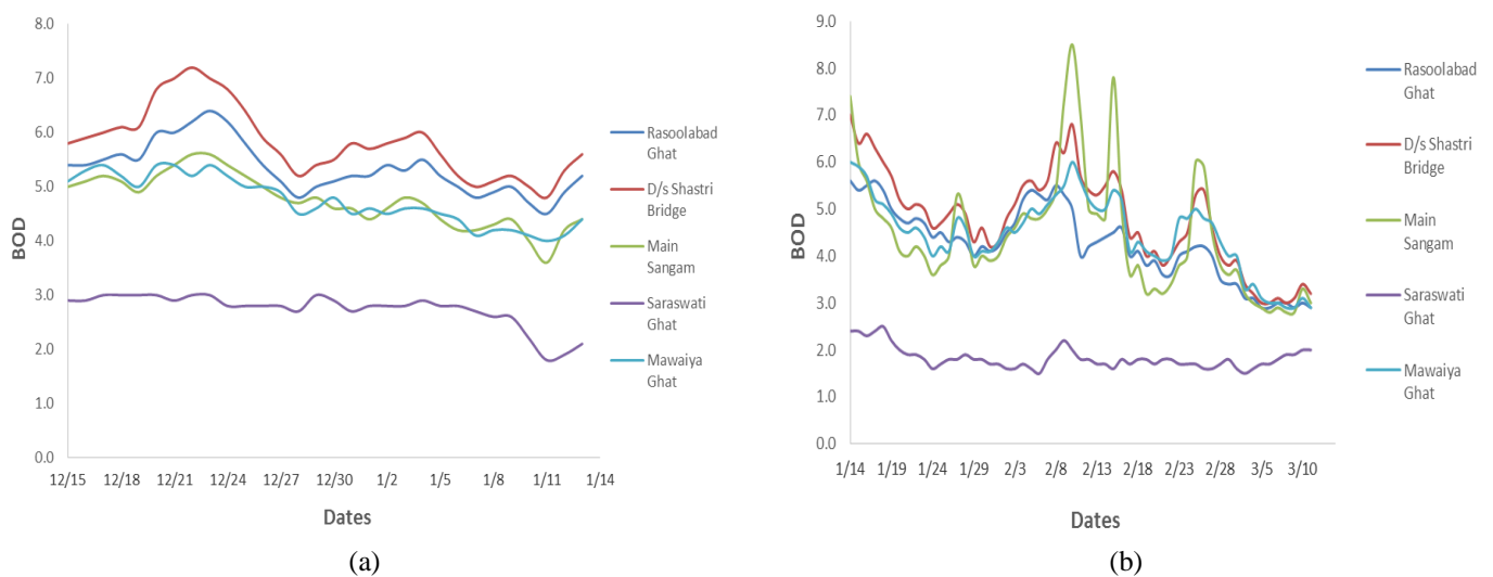
Fig 4: Variation of ‘BOD’ at all the ghats (a) Pre-mela duration, and (b) During the mela
