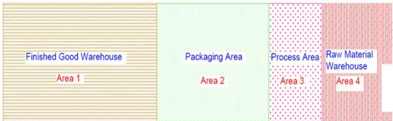
Fig 1 Main Plant Building layout (245 m x 60 m) with demarcation of different functional areas
