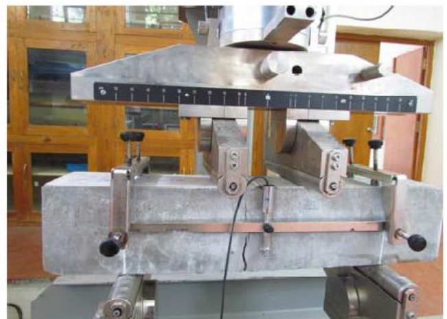
Fig. 2 Loading set-up and yoke fixed to the neutral axis of the prism
