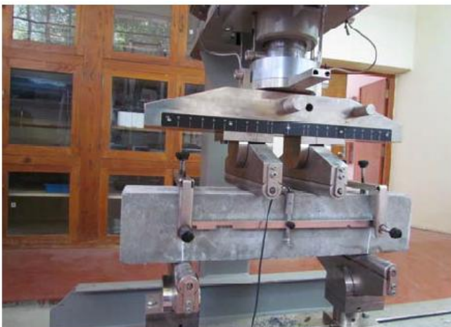
Fig. 2 Loading set-up and yoke fixed to the neutral axis of the prism
