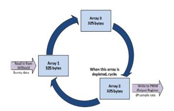
Pulse width modulation works by encoding analog values into a digital square wave by changing its duty cycles. Thus the incoming packets are processed by PWM. The ATMega328p produces music by using this technique. Lower analog frequencies are encoded in a much higher digital frequency and then sent through a low pass filter in order to regain the desired signal.
