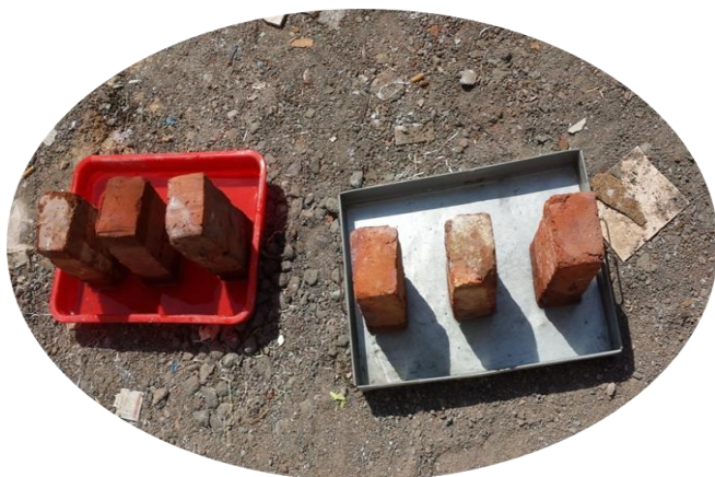
Figure-13: Efflorescence of Various Geo Plastic Bricks
