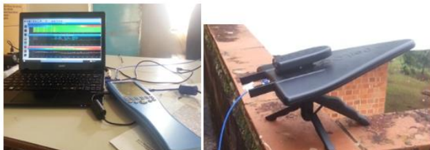
Figure 2 Spectran HF 6065 V4 interfaced to laptop and Antenna on top of the building
