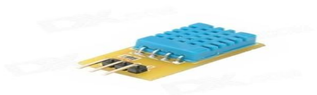
Fig-8: Humidity Sensor
