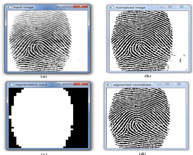
Fig -10: (a) Input image, (b) Normalized image, (c) Segmentation mask, (d) Segmented normalized image
