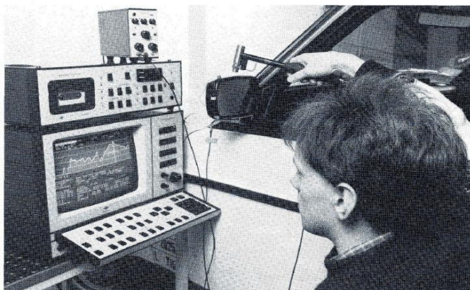
Fig-2: Modal Testing Setup for ORVM
