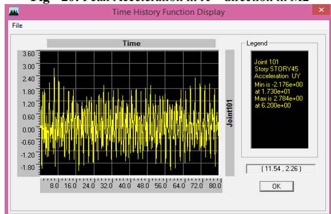
Fig - 21: Peak Acceleration in Y – direction in M2
