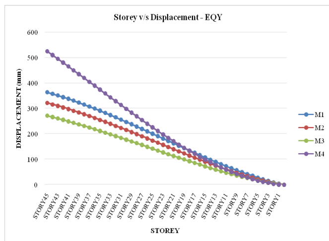
Fig - 9: Storey displacement in x direction for 45 storey seismic analysis
