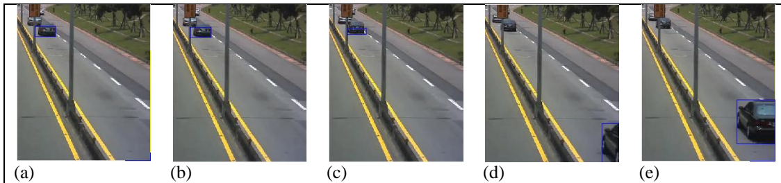
Fig. 4. Detection and tracking of vehicle by kalman filter for an image sequence. Please note that the given sequence is intermediate samples and not temporally interlinked with each other.
