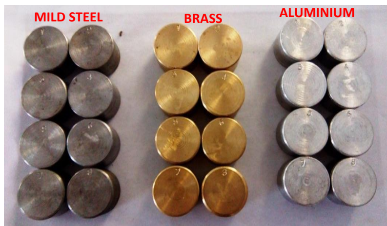
Fig-2: Pool of Work-pieces; extreme left- Mild steel, middle- Brass and extreme right- Aluminium
