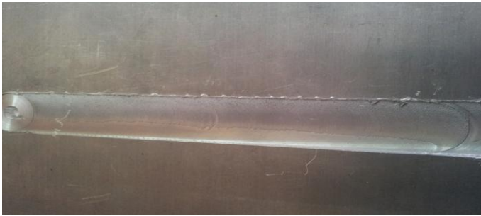
Fig 2.2: Welded plate at 450 rpm
