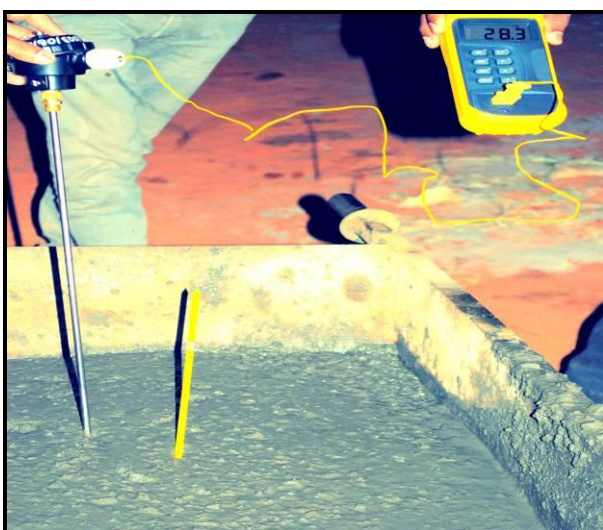
Fig -1: Concrete Placing Temperature
