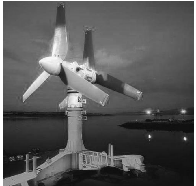
Fig -3: Horizontal axis tidal current turbine [7]
