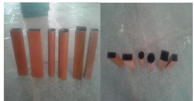
Fig-3: Steel tubes for casting of CFST specimens
