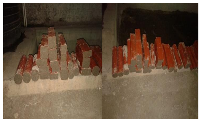
Fig-4: CFST Specimens immediate after casting.
