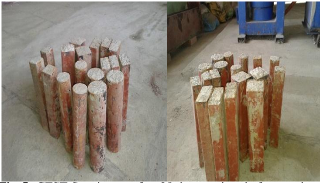
Fig-5: CFST Specimens after 28 days curing, before testing.
