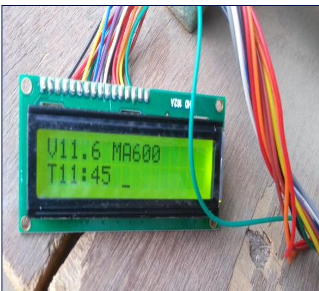
Fig- 13: Different values of voltage and current while tracking the maximum power.
