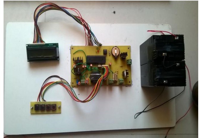
Fig- 8: Hardware Implementation of MPPT(without panel)
