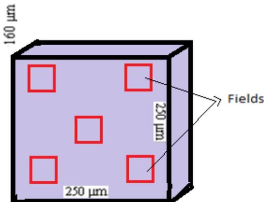
Fig.4. The 5 distinct fields on surface of the material sample marked for acquiring microstructure images using light optical microscope
