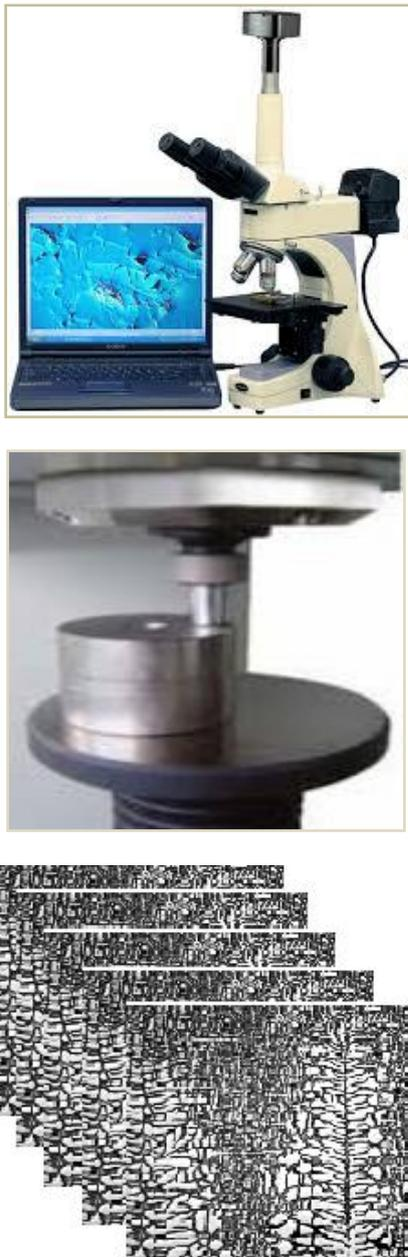
**Fig.1.** Metallography: (a) Serial sectioning machine, (b) Microscope fitted with digital camera-interfaced with computer, (c) Serial sectioned material mounted on microscope and (d) Stack of Serial section images of material.
