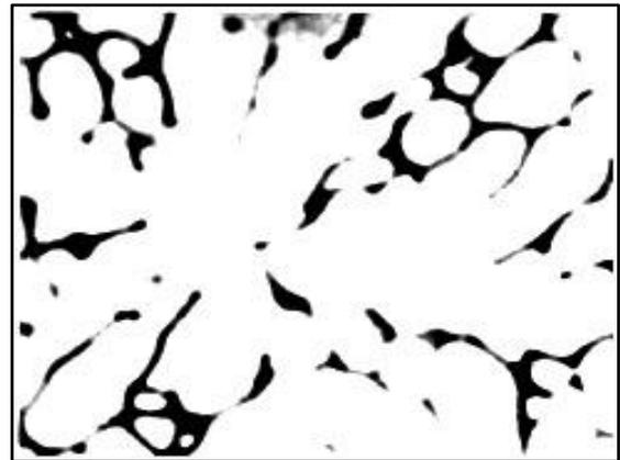
Fig.5: The resultant image after applying filtering by selective median switching filter and Otsu's segmentation methods on microstructure image shown in Fig. 1.
