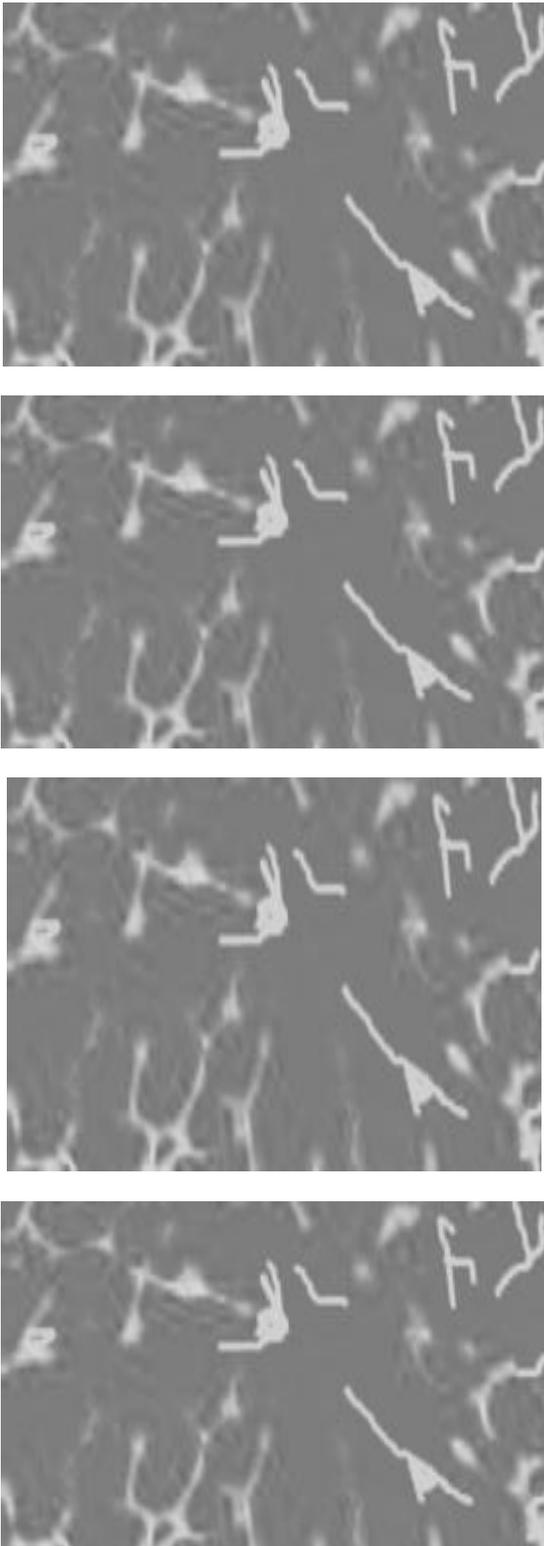
**Fig. 6.** 2D slices showing highly interconnected network of  $\beta$ -Mg<sub>17</sub>Al<sub>12</sub>.
