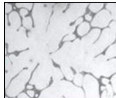
**Fig.2.** Dendrite structures in microstructure image
