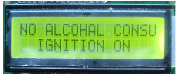
Fig.9.LCD showing no alcohol is consumed by driver
