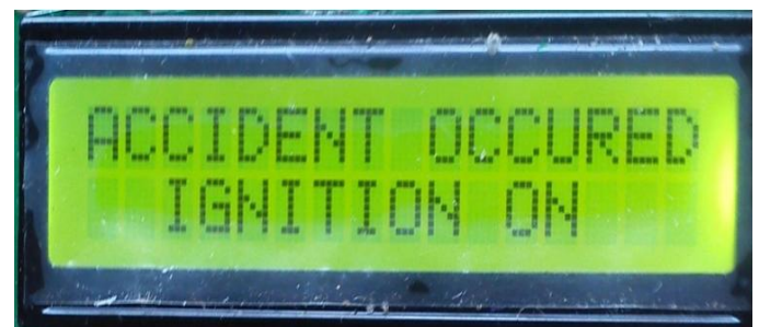
Fig.11.Accident occurred message displayed on LCD
