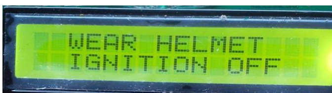
Fig.8. LCD module displaying the message to wear helmet
