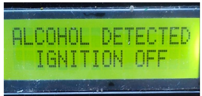
Fig.10.LCD showing alcohol is consumed by the driver
